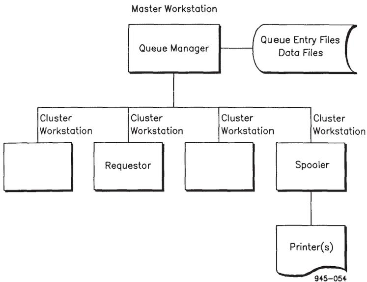
**Figure 35-1. Example of a Configuration with the Queue Management Facility**
