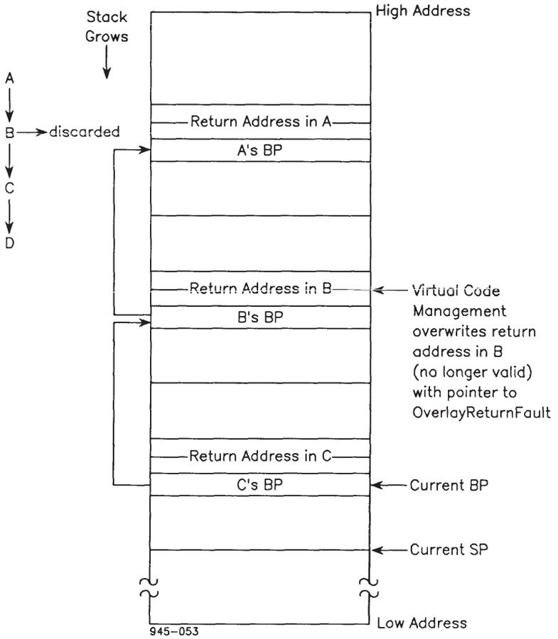
Figure 34-3. Tracing the Stack When an Overlay Is Discarded
