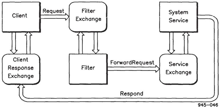
Figure 31-7. One-Way Pass-Through Filter
