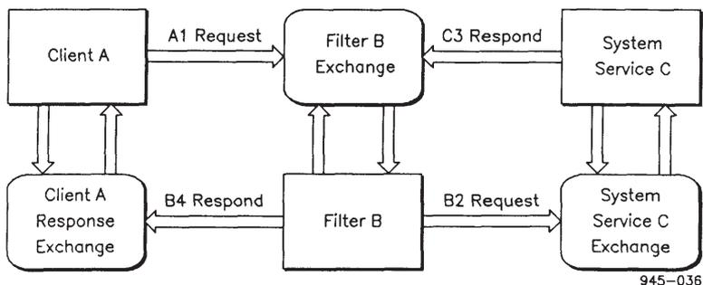
Figure 29-16. Interaction of Filter Process with Client and System Service Process
