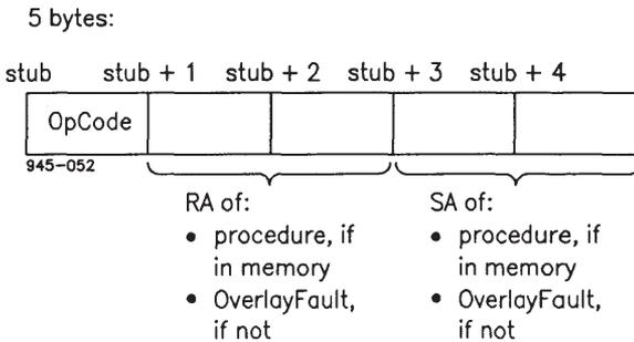
Figure 34-2. Stub Structure
