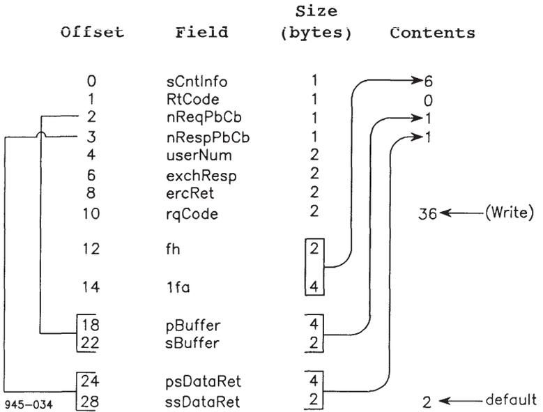
**Figure 29-15. Request Block for the Write Operation**
