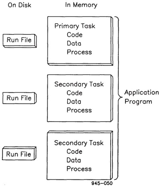
Figure 32-7. Program Consisting of More Than One Run File in an Application Partition
