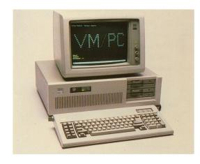
**Performance:** The IBM Personal Computer AT/370, when operating under VM/PC as a CMS machine, executes instructions at 40% to 60% of the speed of a 4331 Model Group 1 doing commercial work and at 1.25 to 2.5 times the speed of a 4331 Model Group 1 performing scientific calculations. Trivial XEDIT commands are performed with less than one second response time
