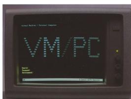
mode, high-resolution color graphics in any 16 colors at one time from a palette of 64 colors in PC mode (640x350 pels), 13-inch screen (measured diagonally)—plus brightness and contrast controls
