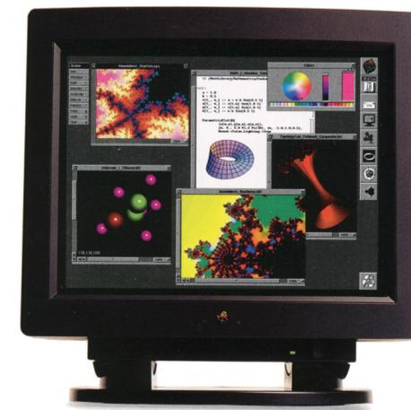
NeXT computers use Display PostScript® for both screen imaging and printing. This makes two key things possible: First, what you see on the screen is precisely what you get when you print. Second, it means that imaging happens in the NeXT computer—not in the printer. So there's no need for the printer to have its own processor. That's why the NeXT 400 dpi Laser Printer is one of the most affordable printers around.
