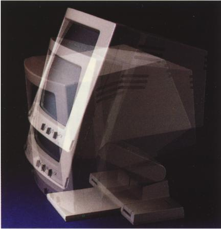
The Explorer system console consists of the monitor, keyboard, and mouse. Connection of the console to the system is through a high-speed fiber-optic link, allowing a flexible lightweight cable of up to 200 feet and providing a transfer rate of 68 megapixels per second.
